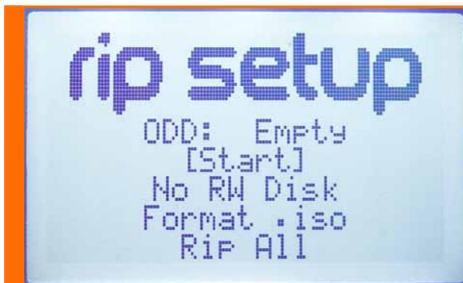
The ISO built from your original disc inserted can be customized trough the settings in the “rip-setup” menu:
