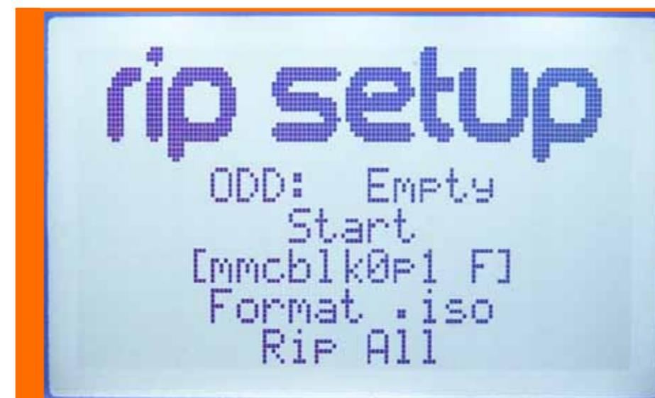
To select the destination device where the backup ISO is stored, you can use the usual screen used to select the mass-storage devices connected; the screen will show only the “writeenabled” devices by WODE.
