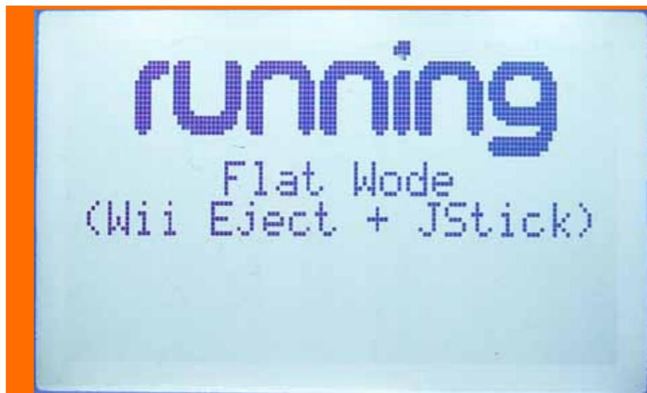
To exit from this mode you have to hold down the WODE-Joystick on any direction and tap the Wii-Eject button. The WODE-Joystick has to be hold down until a message will be displayed on the screen.
