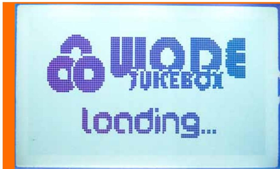
This loading screen is very important, because it confirms that the BOOT LOADER of the WODE is working and is initializing. The boot loader is a micro software that loads the firmware of WODE or – in case the firmware is damaged – it will look for an update file to restore the firmware in the SD/SDHC card slot.
