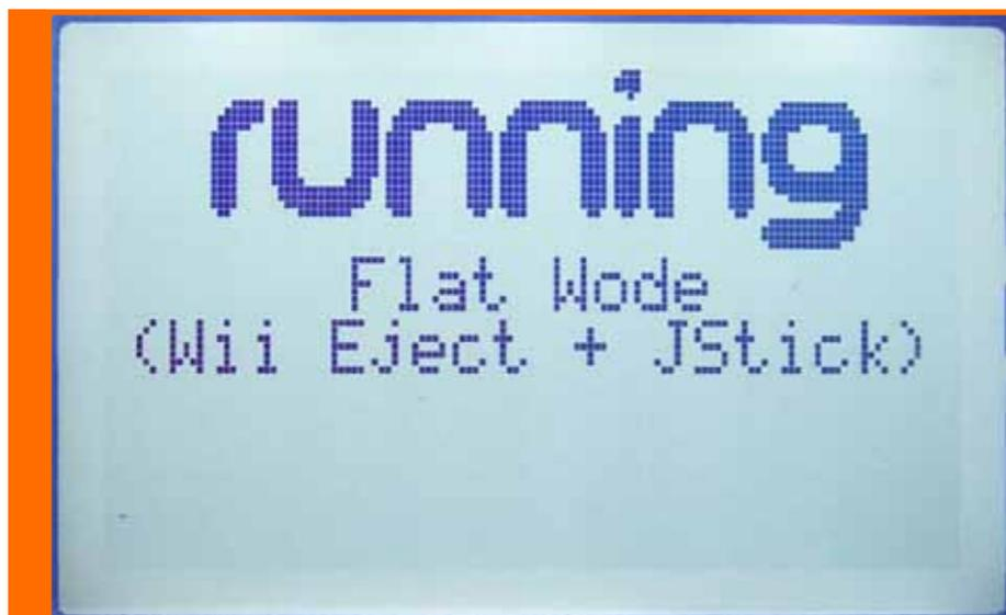
To go back to the main menu, hold down the WODE-Joystick in any direction and tap the Wii-Eject button; hold down the WODE-joystick until the main menu is displayed.
