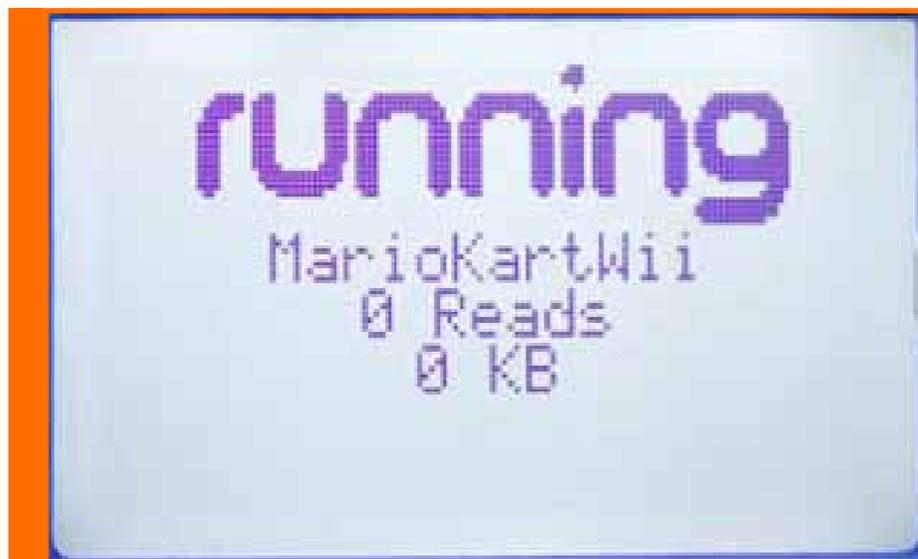
The first line shows the name of the loaded ISO, the second shows the amount of packets transferred , while the third one displays the amount of data transferred in KByte (KB or KiB).
