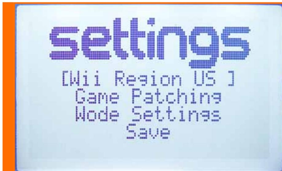
It's important to keep in mind that every setting's modification has to be saved; after having modified the settings, you will have to proceed with saving, selecting the corresponding line and moving the WODE-Joystick to the right.
